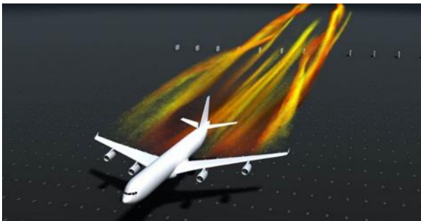
Fig. 1: Numerical simulation of wake vortex evolution generated by landing A340 aircraft with plate line.
