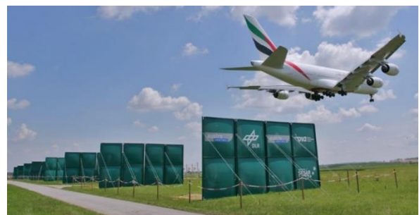
Fig. 3: Overflight of A380 of one of the experimental plate lines installed at runway 16 of Airport Vienna.
