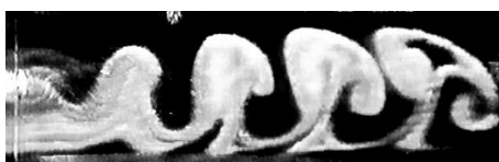
Fig. 1: Visualization of the near vortex street in the region x_1/d = 0-26 .
