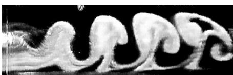
**Fig. 1:** Visualization of the near vortex street in the region  $x_1/d=0-26$ .
